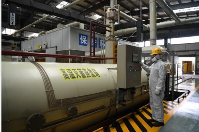
Pic: Medical waste treatment autoclaving plant in city Changsha (near Wuhan) during epidemic, reported by local media.
