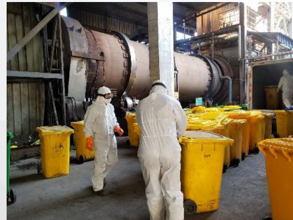
Pic: A rotary kiln treats medical waste in Wuhan. Source: Globaltimes
